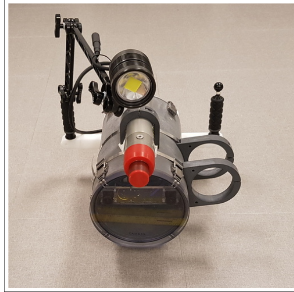
Figure 5.4: Front top view of the assembled sensor suite.
